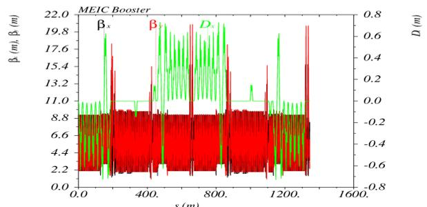
Figure 6: Linear optics of the large booster.
