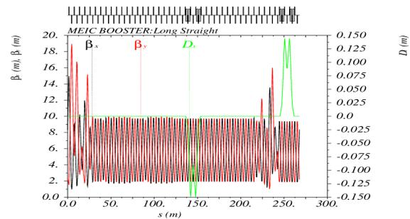
Figure 5: The optics of one of the long straight sections in the large booster.
