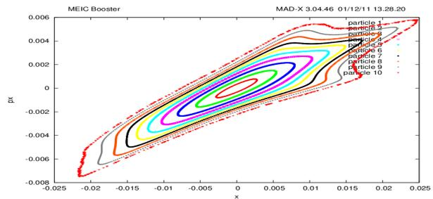
Figure 7: Ten orbits started at 1 through 10 standard deviations radially in horizontal phase space. They are advanced through 1000 turns to examine orbit stability.
