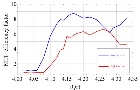
Figure 6: Dependence of the multi turn efficiency factor on the horizontal tune and beam current. Space charge shifts the optimum tune and emittance blow-up reduces the maximum reachable efficiency. Increasing the transverse emittances, shifts the maximum of the MTI efficiency to higher values.
