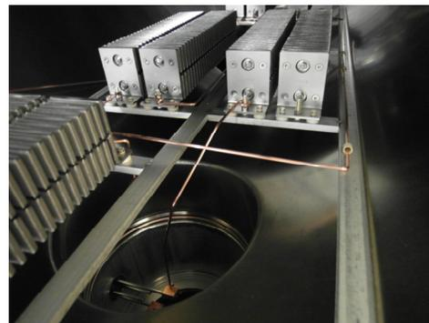
Figure 1: Major ionization beam loss has been caused by pressure bumps in the electrostatic injection septum. To enhance the pumping power and to speed up the recovery process, two sets of NEG panels have been installed in the electrostatic injection septum.
