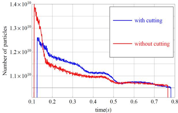
Figure 5: Comparison of the number of ions over a SIS18 cycle with and without injection of a collimated, sharp edge ion beam. With injection of a trimmed beam, the same number of ions can be achieved at extraction with a significantly lower number of ions injected.
