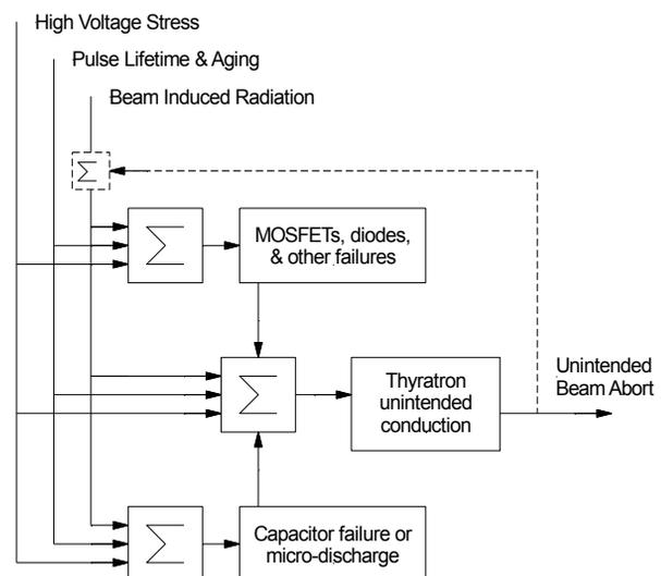
Figure 1: Main factors contributing to unintended beam abort in RHIC beam abort systems.
