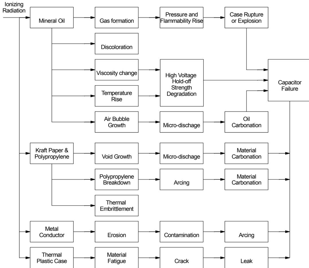
Figure 2: A diagram of possible radiation effects on oil filled capacitors.
