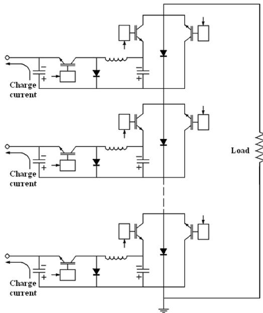
Figure 3: New topology for Marx modulators.
