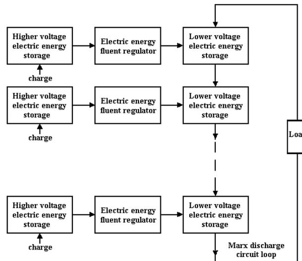
Figure 1: Diagram for designing a new Marx modulator.
