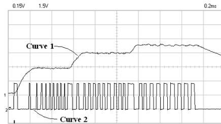
Figure 5: Terrace voltage pulse output by the new Marx.
