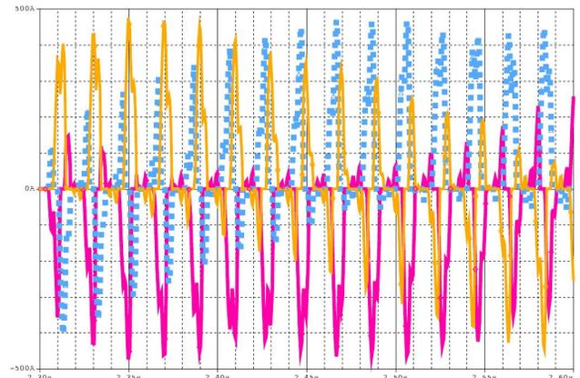
Figure 2: Spice simulation of the basic SMPS showing currents drawn from each phase of the AC supply.
