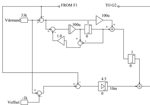
Figure 3: Spice model of the new inhibit control loop.
