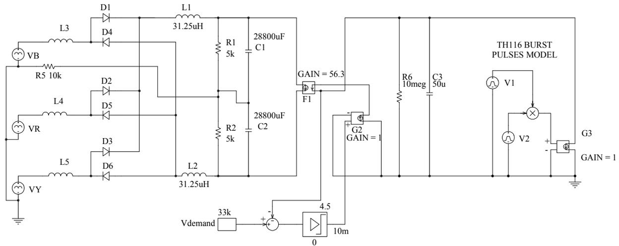
Figure 1: Simplified SPICE model of 4 switch mode power supplies parallel connected.
