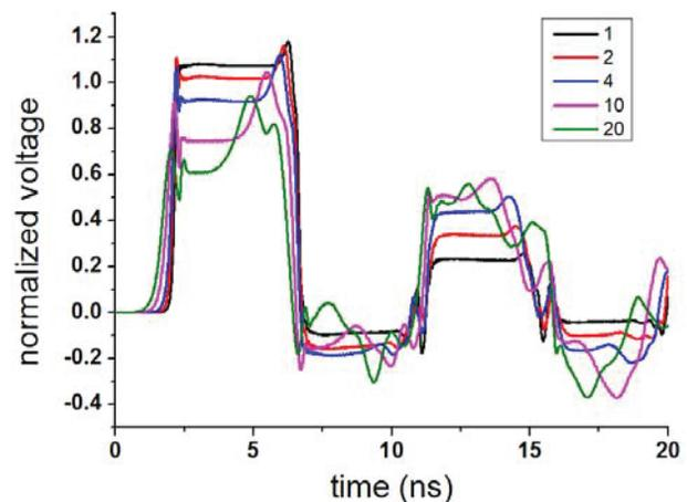
Figure 4: Normalized output pulses for stacked-Blumlein with different number of Blumleins.
