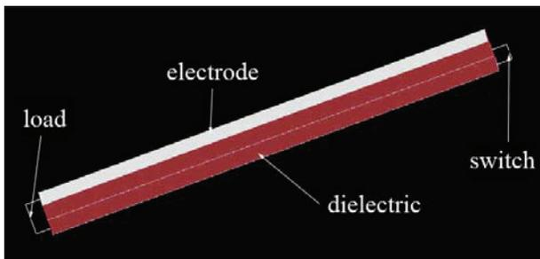
Figure 1: Model of a parallel-plate Blumlein.
