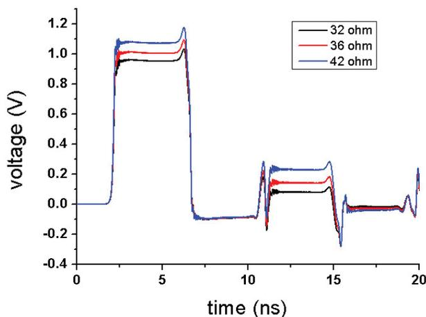
Figure 3: Output pulses on a resistive load with various resistances.
