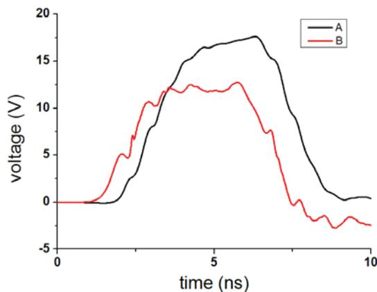
Figure 7: Output pulse across the HGI, A - 2 mm gap between adjacent Blumleins, 0.4 ns turn-on time of switches; B - no gap between adjacent Blumleins, 20 ps turn-on time of switches.
