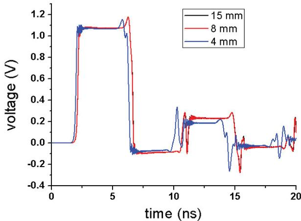
Figure 2: Output pulses for a 4-mm-wide Blumlein with different dielectric widths
