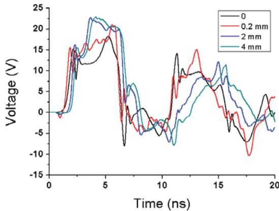
Figure 5: Output pulses with different adjacent Blumlein separations.
