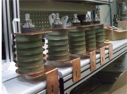
Figure 4: The assembled discharge resistor sets.
