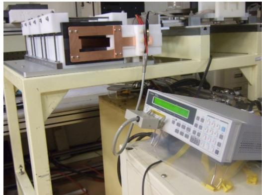
Figure 5: The standard inductive load.
