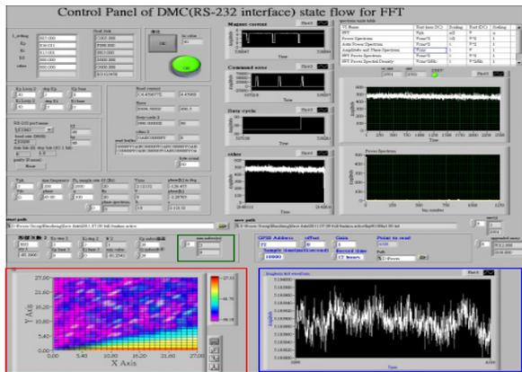
Figure 2: The virtual instrument control interface of digital regulation power supply.
