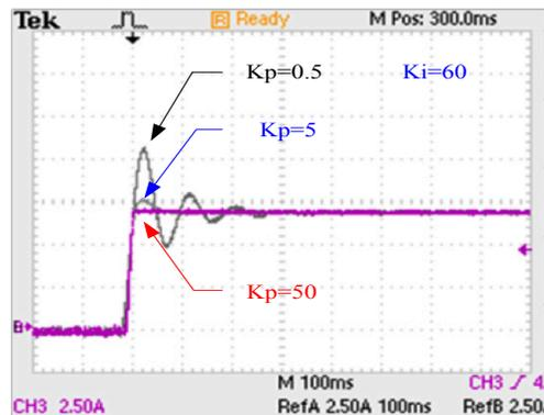
Figure 3: The step response of power converter.
