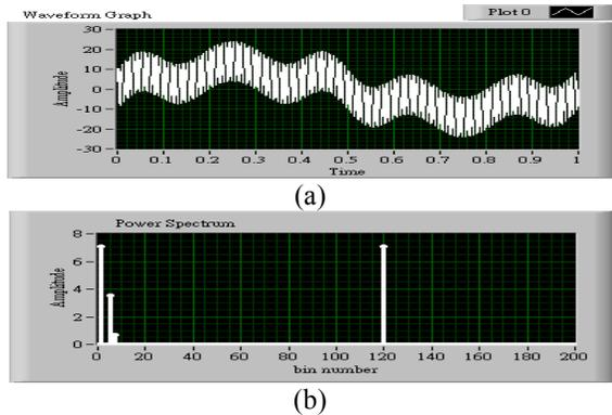
Figure 6: The FFT analysis (a) Capture in the LabVIEW, (b) Spectrum of waveform.
