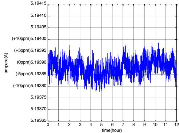
Figure 8: Stability of output current of power converter.
