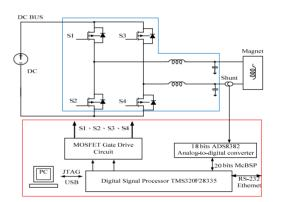
Figure 1: The structure of corrector magnet power converter.
