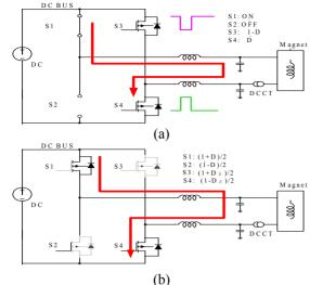
Figure 2: The operation of switching pattern (a) one arm (b) pair arms.
