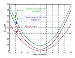
Figure 7: Input and output of power converter.
