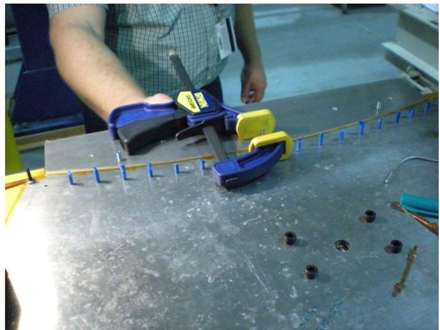
Figure 5: Conductor being held in place in negative curvature section of the coil while epoxy is drying.
