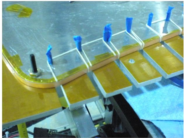
Figure 4: Winding YBCO coil with inverse curvature segment using Kevlar string to hold the conductor in place.
