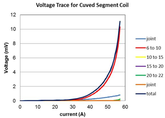
Figure 7: V vs. I trace for the coil with the curved inner segment.
