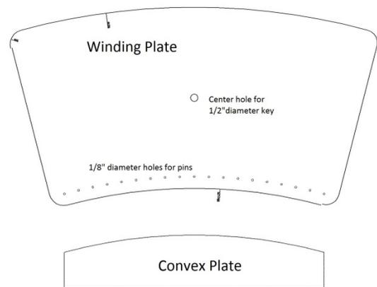
Figure 2: Winding tools used to wind coil with concave segment.
