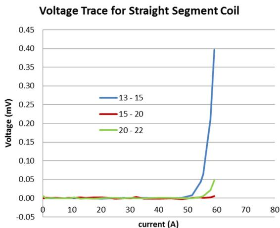
Figure 6: V vs. I trace for the coil with the straight inner segment.
