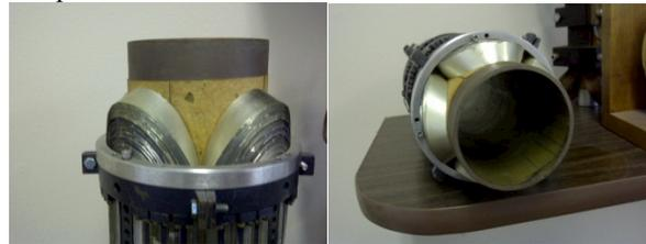
Figure 3: Photograph of coil ends of a test quadrupole wound with Nb<sub>3</sub>Sn tape.
