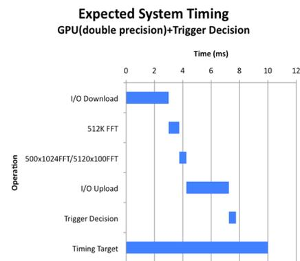
Figure 3: Details of GPU benchmark timing assuming Correlate/Max is performed on GPU (double precision). Splitting the trigger algorithm implementation across multiple CPU cores can further optimize the time taken to make the trigger decision.
