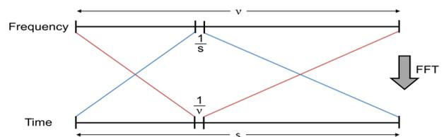
Figure 1: The relationship of the frequency domain data and the time domain data. The time domain data can be calibrated to provide data as a function of length. The length data is then used to create the distributed measurement segments that can be used for quench detection (figure taken from [5]).
