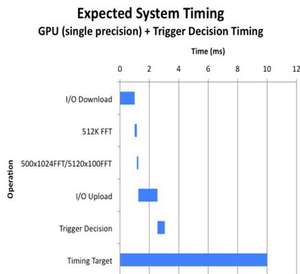
Figure 4: Details of GPU benchmark timing assuming Correlate/Max is performed on GPU (single precision). One can see using single precision provides significant performance gains over the use of double precision.
