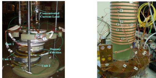
Figure 5: 3 T, six coil, short section of helical solenoid (YBCO). (left) and a test coil with fibers and quench heaters (right).
