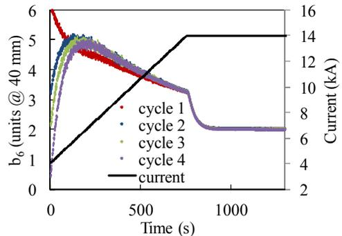
Figure 7: Repeatability of  $b_6$  measurements in four excitation cycles. The multipole depends on the pre-cycling conditions at low field but it is repeatable at nominal field.
