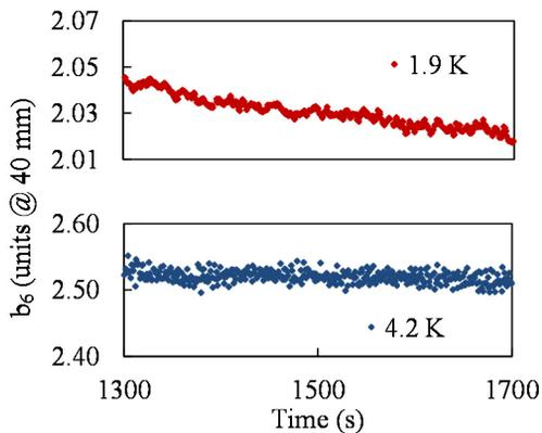
Figure 5: Precision of  $b_6$  measurements during a plateau at nominal current level. Both for operation at 1.9 (red) and 4.2 K (blue).
