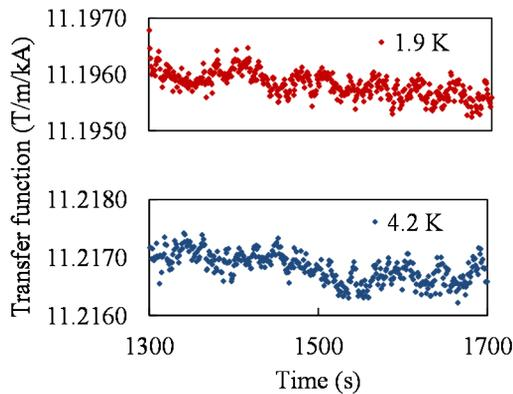
Figure 4: Precision of transfer function measurements during a plateau at nominal current level. Both for operation at 1.9 (red) and 4.2 K (blue).
