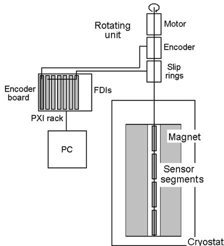
Figure 2: Schematic of the measurement system.
