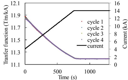
Figure 6: Repeatability of transfer function measurements in four excitation cycles.
