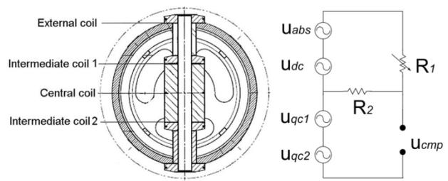
Figure 1: Left: Cross-section of the measurement shaft with search coils. Right: Compensation scheme for the induced voltages in the search coils.
