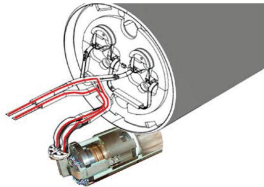
Figure 3: dipole bypass path; the red line indicates the flow of current in case of a quench.
