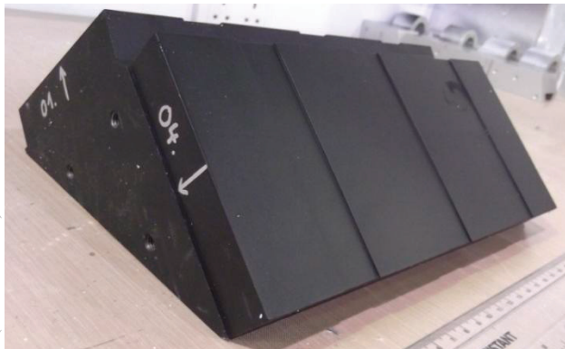
Figure 5: One of the two assemblies of PMs and steel wedge, prior to assembly into the quadrupole.
