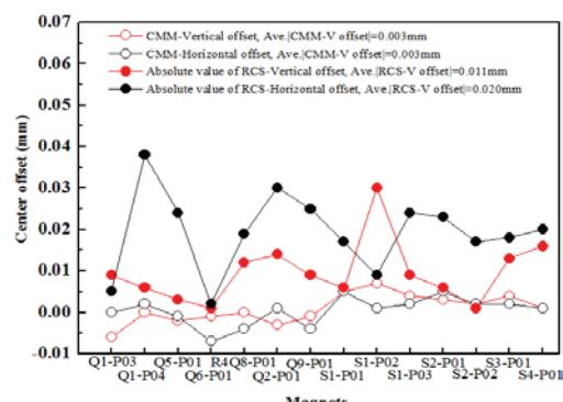
Figure 3: Center offsets of multipole magnets measured with the CMM and RCS.
