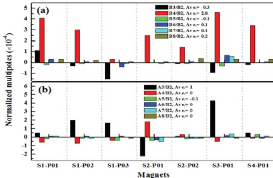
Figure 6: (a) Normalized normal (b) skew multipole of sextupole magnets.
