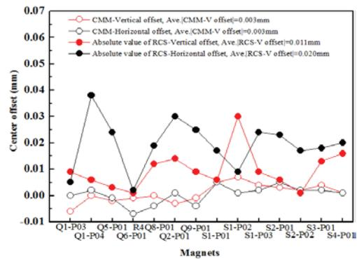
Figure 3: Center offsets of multipole magnets measured with the CMM and RCS.
