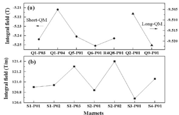
Figure 4: Integral field of (a) quadrupole and (b) sextupole magnets.
