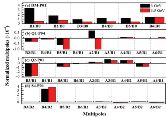
Figure 7: Normalized multipoles of (a) DM-P01, (b) Q1-P04, (c) Q2-P01 and (d) S4-P01 in 3-GeV and 3.5-GeV conditions.
