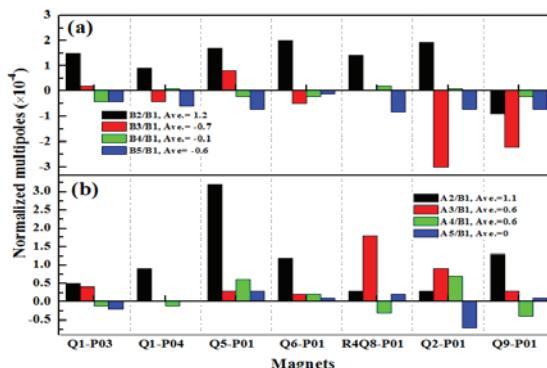
Figure 5: (a) Normalized normal and (b) skew multipole of quadrupole magnets.
