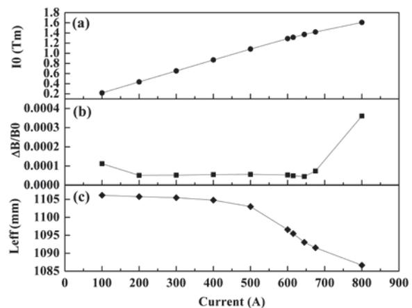
Figure 1: (a) integral IB-curve, (b) field homogeneity of the center line and (c) effective length of a DM-P01 magnet which is as a function of the excitation current.
