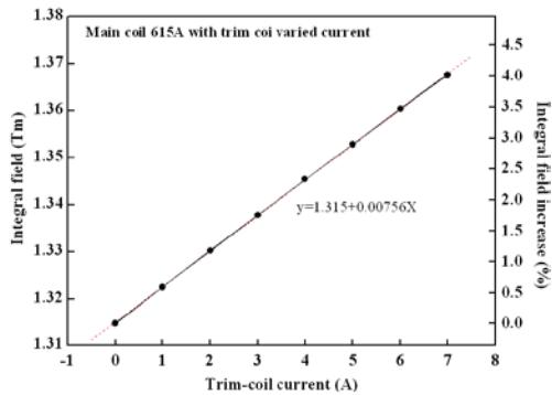
Figure 2: Integral combination-field from combining main and trim coils of a DM-P01 magnet. The left and right axes display the integral field and field-increase ratio, respectively.
