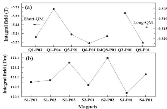
Figure 4: Integral field of (a) quadrupole and (b) sextupole magnets.
