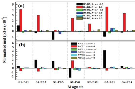
Figure 6: (a) Normalized normal (b) skew multipole of sextupole magnets.
