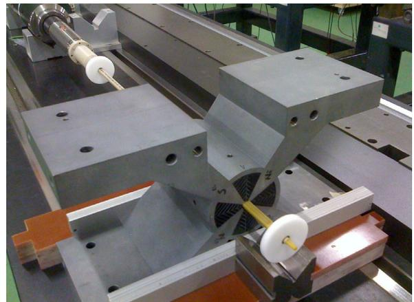
Figure 6: Rotating coils measuring system (7.7 mm diameter) under commissioning at CERN.
