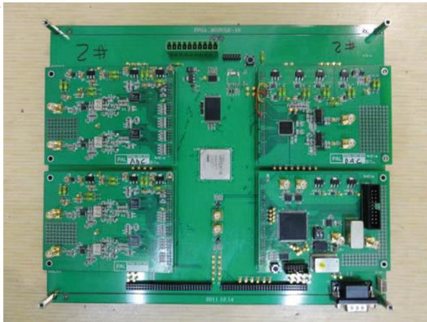
Figure 3 : Printed circuits board for the LLRF system: Left two daughter boards are the ADC, right upper board is DAC, right bottom is the clock generator and digital input and output and two connectors at bottom are spare for the other functions.
