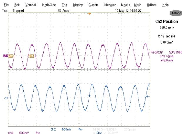
Figure 4 : DDS output signals of the sine and cosine function corresponding to I and Q.
