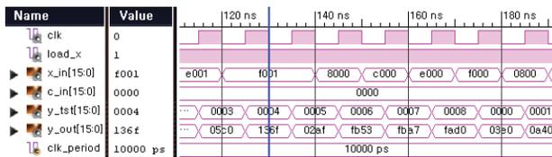
Figure 7 : FIR filter simulation using the ISIM.
