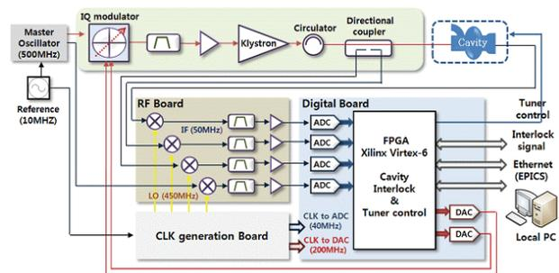
Figure 1: Block diagram of the LLRF system for PLS-II.
