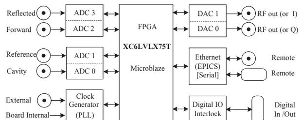
Figure 2 : Block diagram of the designed FPGA with peripheral devices.
