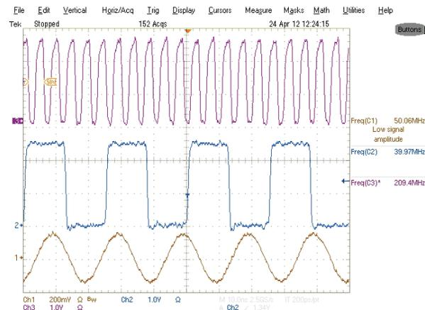
Figure 5: Signals generated by the Spartan6 for DAC, ADC and IF.
