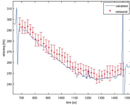
Figure 1: Detuning calculated with eq. (3) and measured with shortening RF pulse. Red bars - results of measurements (with RMS error), blue line - result of calculations.
