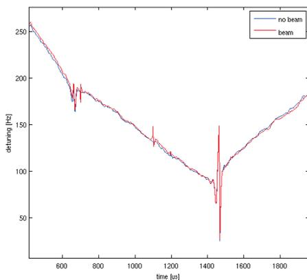
Figure 4: Detuning calculation using the formula (3) with beam contribution. Blue - no beam condition. Red - with beam
