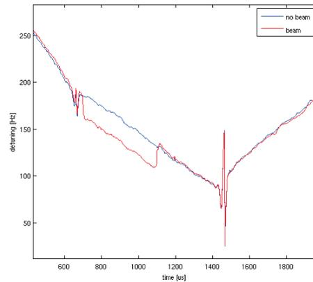
Figure 2: Detuning calculation for no beam conditions (blue) and beam condition (red) without taking into account the beam contribution. The beam current was 4.5mA with 1200 bunches (beam was present between 700 $\mu$ s and 1100 $\mu$ s)
