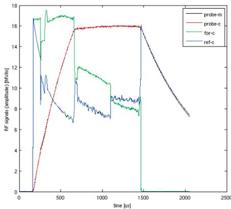
Figure 3: RF signals with beam. Both measured and calculated cavity voltage fits well that indicates the good calibration of the RF signals.
