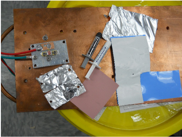
Figure 5: Cooling experiment. Tested materials include: Indium foil, Aluminium foil, Sil-Pad 900S film, Sil-Pad 2003 film, Thermal compounds.
