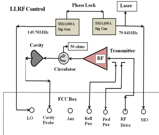
Figure 5: LLRF system block diagram.
