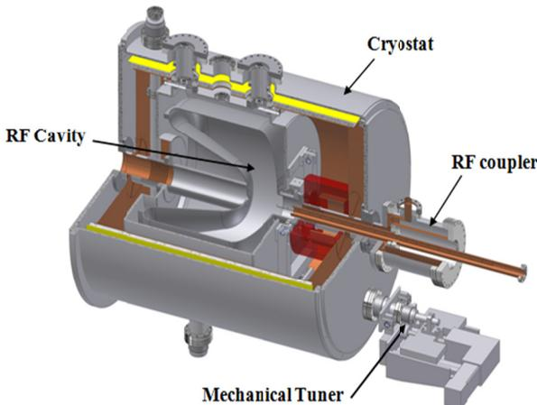
Figure 3: Superconducting RF electron gun.
