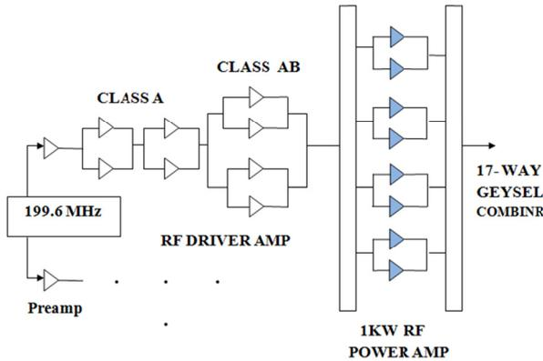
Figure 2: Block diagram of RF amplifier chain.
