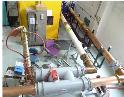
Figure 3: High power coaxial hybrid in test.
