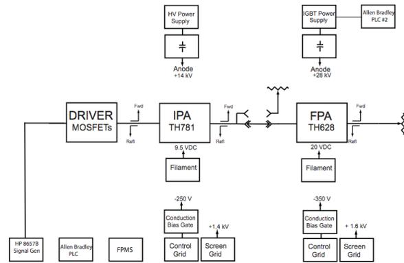
Figure 1: Block diagram of test arrangement.
