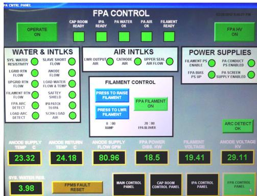
Figure 4: FPA controls in Panelview.
