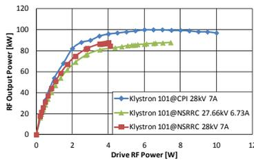
Figure 4: The comparison of drive/output power curves of klystron SN101 between NSRRC and CPI.
