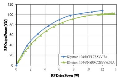
Figure 7: The comparison of drive/output power curves of klystron SN104 between NSRRC and CPI.
