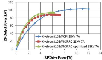
Figure 6: The comparison of drive/output power curves of klystron SN103 between NSRRC and CPI.
