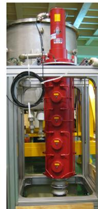
Figure 1: The CPI 100kW klystron on the supporter.
