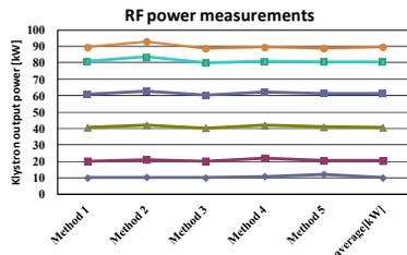
Figure 3: the power balance for RF power calibration of the klystrons.
