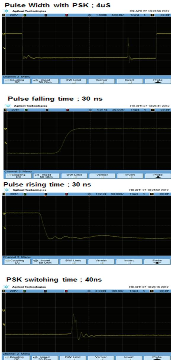
Figure 7: Test results of SSA for ATF
