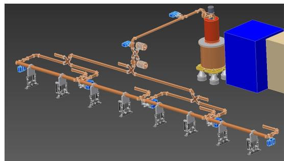
Figure 2: Layout of one klystron module.
