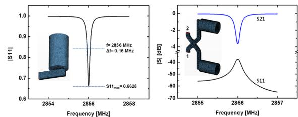
(a) Dual iris coupling (b) SLED with 3 dB hybrid
