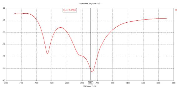
Figure 6: Simulated results of SiC load.
