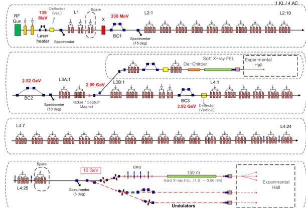
Figure 1: Schematic diagram for the PxFEL.
