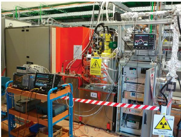
Figure 3: X-band power plant under test on water loads.
