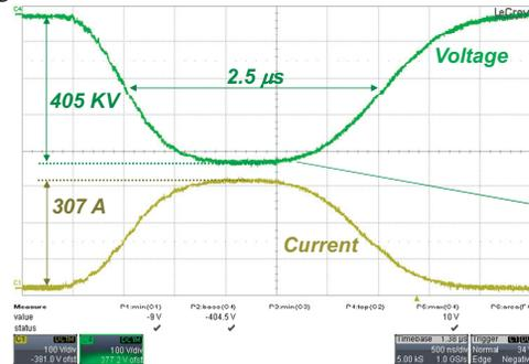
Figure 4: Klystron V-I pulses at 405 KV-307A.
