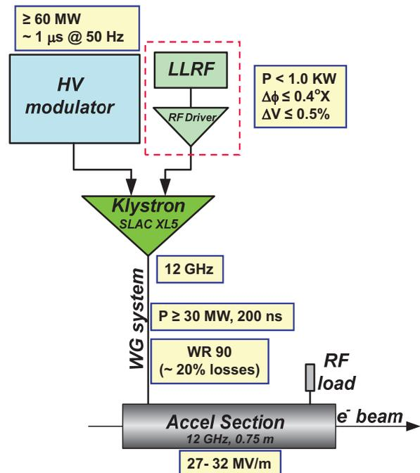
Figure 2: X-band plant layout and main requirements.
