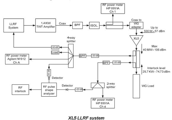
Figure 5: LLRF drive system and power measurement.
