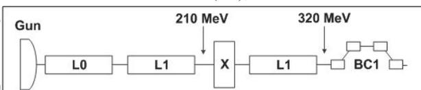
Figure 1: Machine layout up to the first bunch compressor.
