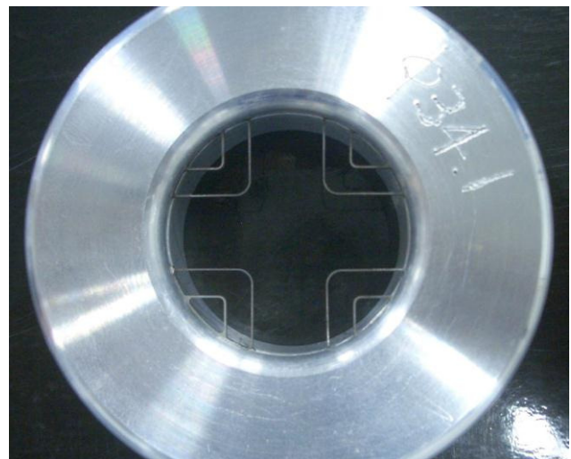
Figure 3: The grid in a mockup drift tube.
