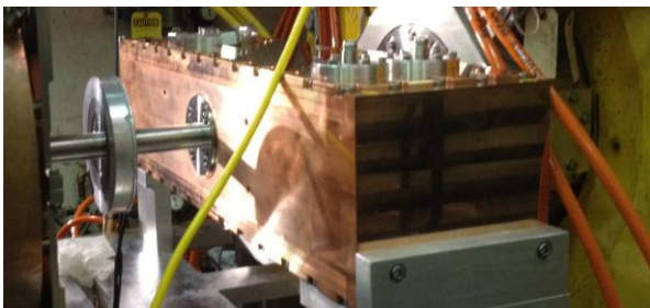
Figure 1: The new copper buncher.
