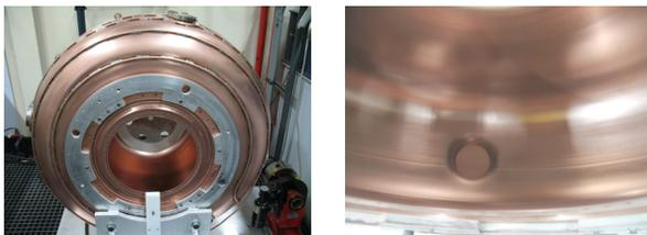
Figure 4: The cavity surface finishing after EP.
