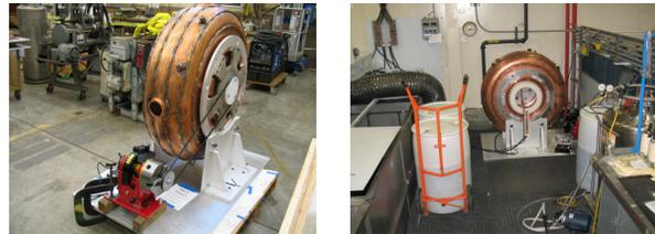
Figure 1: EP Setup. The left figure shows the ventilation side of EP setup, with the pulley, driving belt and rotating motor. It is covered by a ventilation hood during EP. The right figure shows the whole EP setup in the LBNL plating shop.
