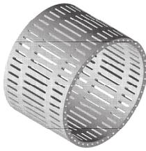
Figure 2: Isometric view of PWT sieve with segmented slots.
