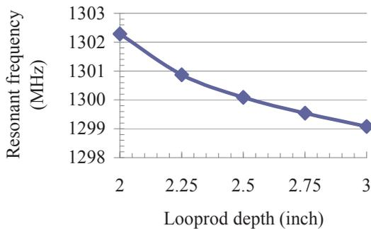
Figure 8: PWT cavity resonant frequency vs probe (looprod) depth.
