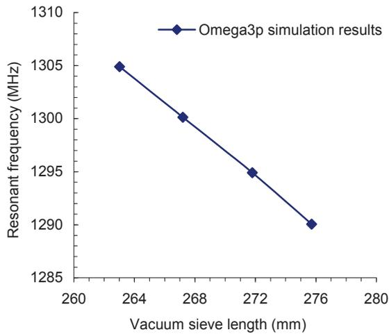
Figure 6: PWT cavity tuning sensitivity from Omega3p code.
