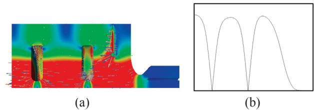
Figure 9: PWT 2-cell gun electric field distribution (a) and field magnitude vs axial distance (b) without sieve from Omega3p code.
