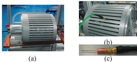
Figure 3: Pictures for cold test model (a) Set up for cold test; (b) A probe is placed through the vacuum sieve slot; (c) A field probe.
