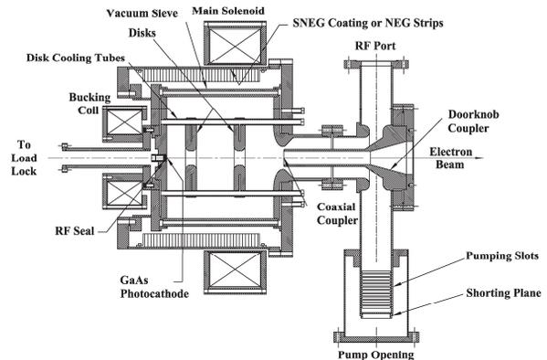
Figure 1: Schematics of an L-Band PWT polarized electron photoinjector.
