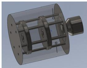
Figure 7: L-Band 2-cell PWT gun model with two probes.
