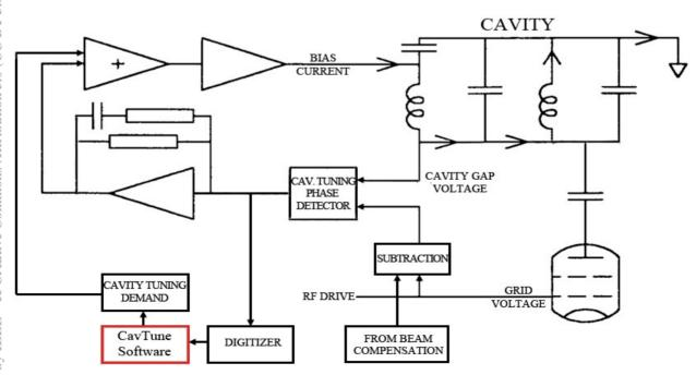
Figure 1: Block diagram of the ISIS Cavity tuning systems.
