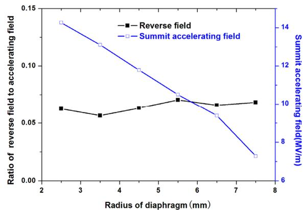
Figure 6: Reverse and accelerating field as a function of the diaphragm's radius.
