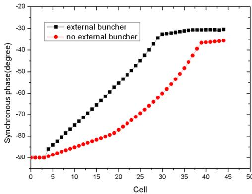
Figure 3: Synchronous phase variations along the RFQ cell number.
