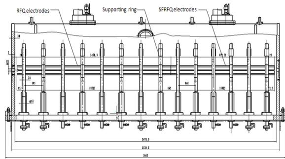
Figure 5: The sketch layout of the coupled RFQ-SFRFQ cavity.
