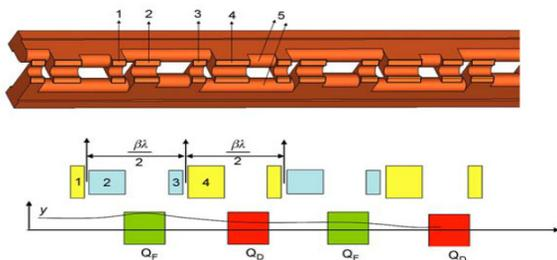
Figure 1: The principle of the SFRFQ (the particles are accelerated between 1&2 and 3&4, focused between 2&3;  $Q_F$  and  $Q_D$  represent the focusing and defocusing lens, respectively).
