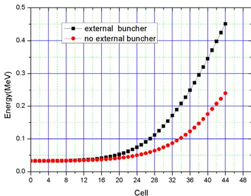
Figure 4: The energy gain of RFQ as a function of cell number.
