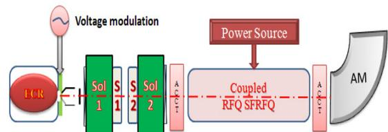
Figure 2: The schematic layout of the accelerating system.
