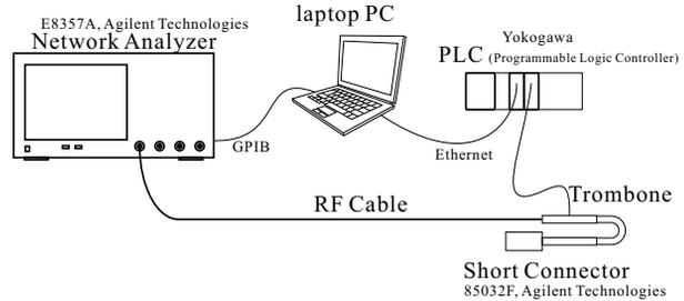
Figure 1: Approach using a network analyzer and a trombone. The trombone was automatically moved and data were taken using the Programmable Logic Controller(PLC) system and the laptop PC.
