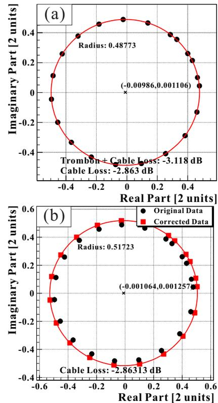
Figure 2: Fitting results of the measurement of the cable attenuation using the trombone. (a) shows the fitting result of the original data. The contribution of the trombone was subtracted after that. The red closed squares of (b) represent the corrected data. The final results of the both corrections were almost the same.
