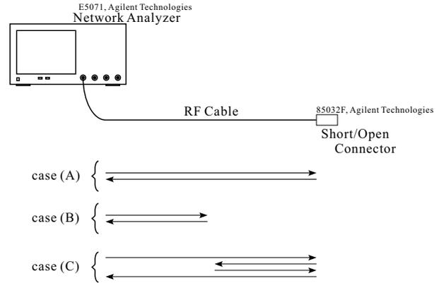
Figure 3: Approach using a network analyzer and connectors. If the reflected wave using a short connector is subtracted from that using an open, the components of case(B) and (C) disappear and the contribution of case(A) is rest.
