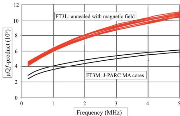
Figure 6: Comparison of FT-3L and FT3M. FT-3L cores achieve higher  $\mu Qf$ -products.
