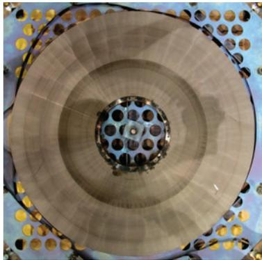
Figure 5: FT-3L core just after annealing under an axial magnetic field. (OD 800 mm × ID 245 mm × t 25 mm.)
