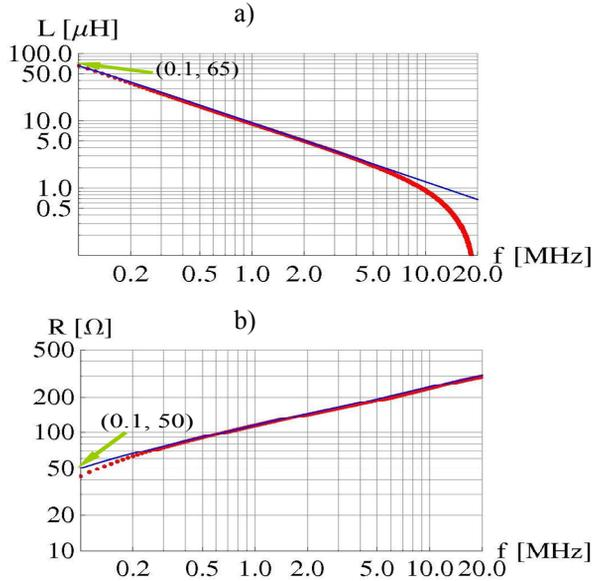
Figure 6: The analytical approach (blue curve) and the measurements in the frequency region from 0.1 to 20 MHz. a) for series inductance L, b) for resistance R
