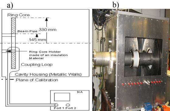
Figure 4: a) Schematic of the setup for measuring the impedance of one ring, mounted in a metallic box. b) BB test cavity under-construction in RF lab at GSI.
