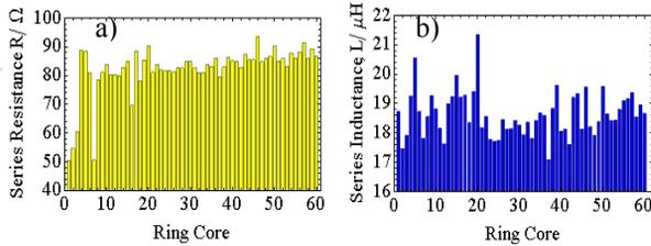
Figure 3: a) R and b) L of all the rings at 0.4 MHz.
