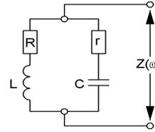
Figure 5: Equivalent circuit to include stray fields.
