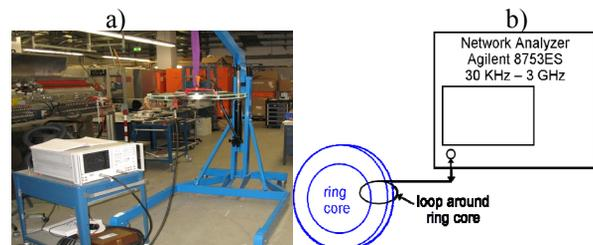
Figure 2: a) Experimental setup and b) a schematic for the ring core measurements in free space.
