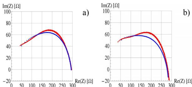
Figure 7: Comparison of the impedance measurement with the analytic approach for left and right rings.
