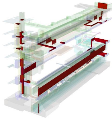
Figure 3: Clash check in the central injector building.
