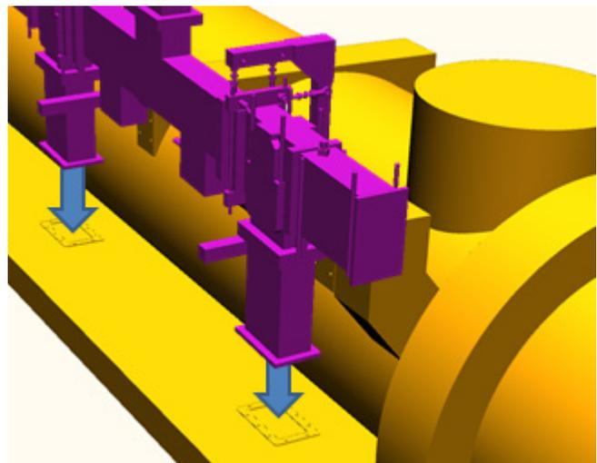
Figure 4: Interface definition with placeholder models.
