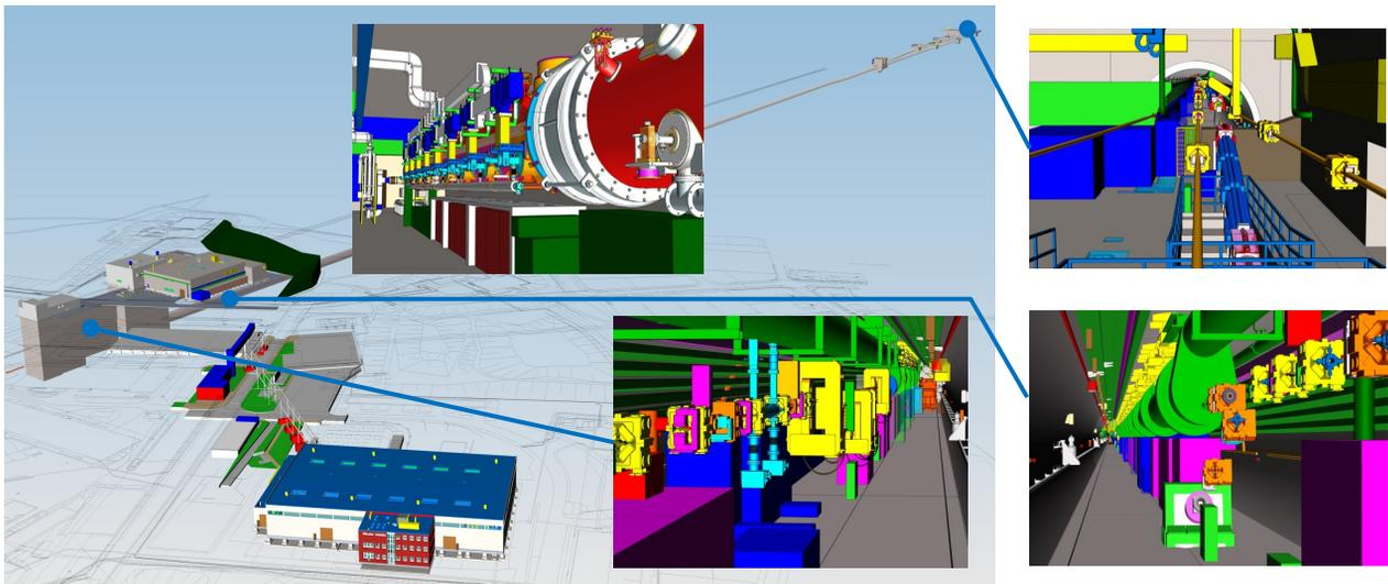
Figure 1: 3D CAD model enabling the project team to interactively explore any region of the facility. The model assembles more than 170,000 parts, color-coding is applied for quickly identifying the different sub-systems.
