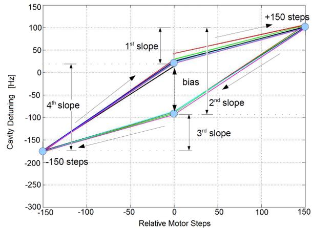
Figure 2: Backlash measured on frequency tuners.
