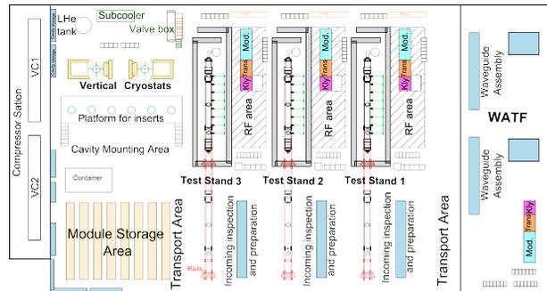
Figure 1: Floor plan of the AMTF hall.
