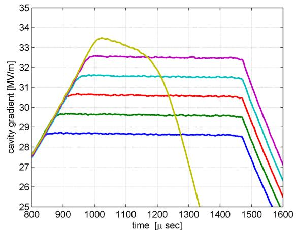
Figure 3: Quench threshold identification.
