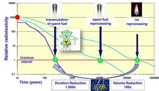
Figure 1: Schematic overview of the nuclear waste problem
