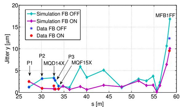
Figure 2: Position jitter propagation for bunch 2 along the ATF extraction line. The simulation predictions are compared with measurement data for the cases FB OFF and ON.
