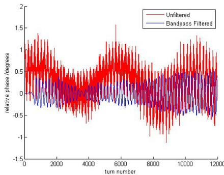
Figure 3: Comparison of unfiltered (red) and band-pass filtered (blue) data for bunch 1. The bursting nature of the synchrotron oscillation can be seen clearly in the filtered data.
