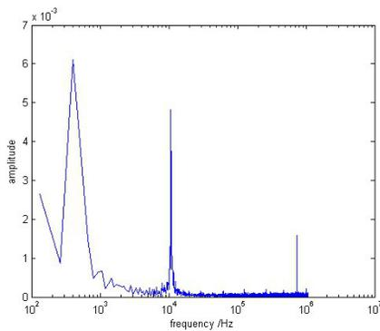
Figure 2: Fourier transform of the relative phase of bunch 1. Bunches 2 and 3 show very similar behaviour.
