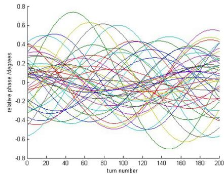
Figure 4: Last 200 turns (one synchrotron period) before extraction for band-pass filtered data for bunch 1. Data for 43 successive pulses is overlaid, showing that the phase of the bunch at extraction is random.
