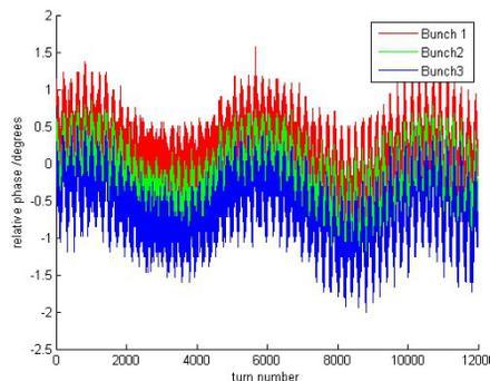
Figure 1: Bunch phase with respect to the LO, for the last c. 12000 turns before extraction for three bunches separated by 154 ns.
