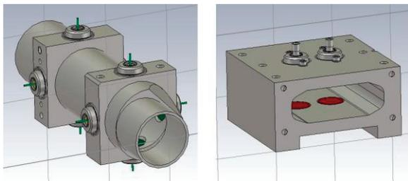
Figure 1: CST renderings, a) cylindrical beampipe section; b) rectangular beampipe section.
