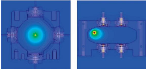
Figure 2: Potentials in the transverse plane: a) cylindrical pickup arrangement, b) rectangular pickup arrangement.
