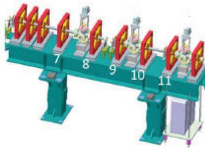
Figure 1: ALICE Tomography Section, indicating quadrupole numbers (7-11).
