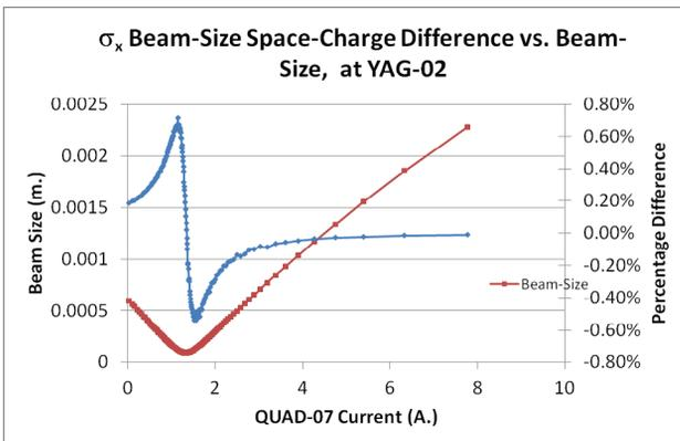
Figure 5: Percentage horizontal change & beam-size at YAG-02, with increasing QUAD-07 current.
