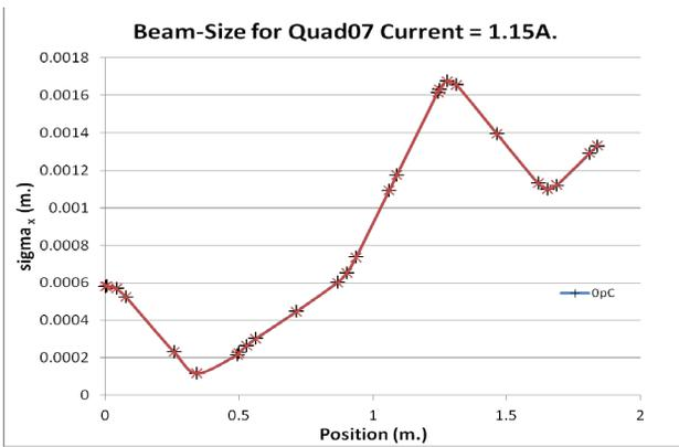
Figure 4: Horizontal RMS beam-size along the tomography beam-line.
