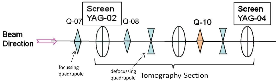
Figure 2: Schematic of ALICE Tomography Line, showing YAG screens and quadrupole magnets.
