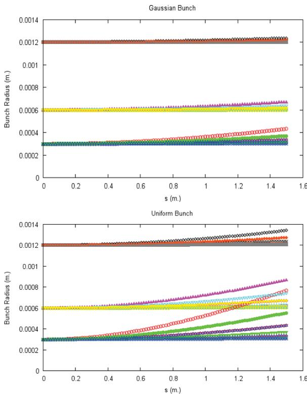
Figure 3a: Analytical Code. Space-charge effect on bunch radius - Gaussian (top) and uniform (bottom).
