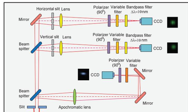
Figure 1: Schematic layout of the beam profile monitoring system.
