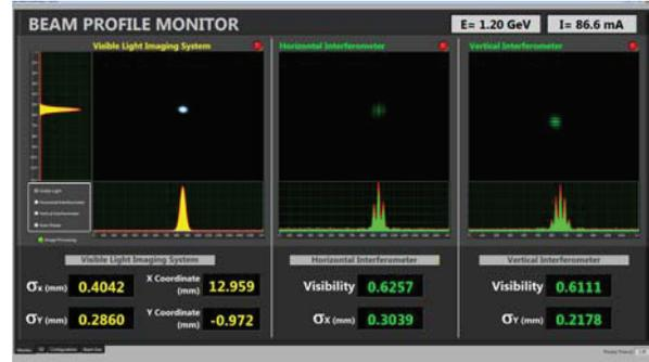
Figure 2: Real-time beam size monitoring panel. The leftmost panel shows the result from the direct imaging system. The two other panels show the results from the SR interferometers.
