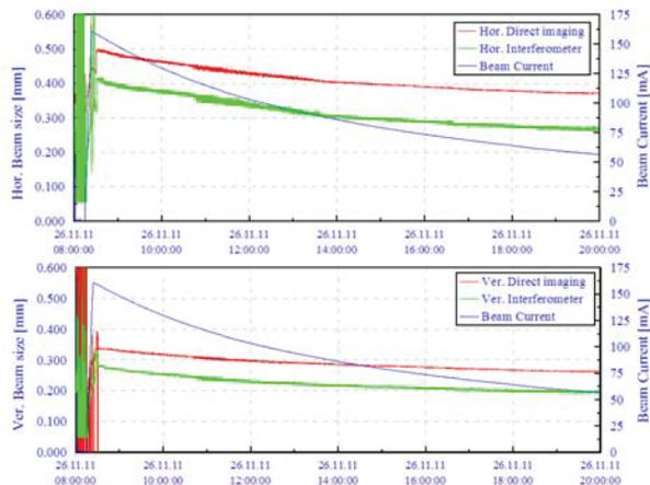
Figure 3: Measured beam sizes from direct imaging and interferometer systems as a function of beam current.
