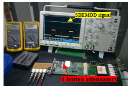
Figure 4: The measurement setup for the calibration of the BPM electronic modules.
