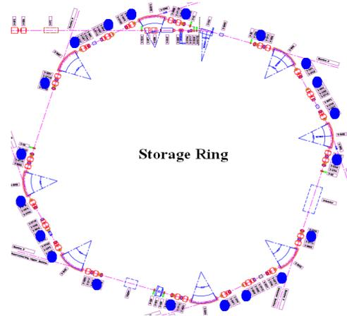
Figure 1: The location of 20 BPMs in the SPS storage ring, indicated by filled circles.
