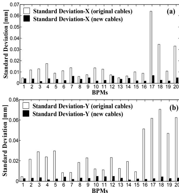
Figure 6: The bar plot of the standard deviations before and after BPM cable replacement.
