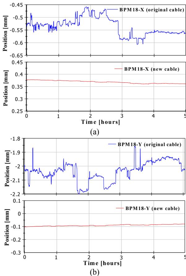
Figure 5: The BPM no. 18 reading during machine operation.
