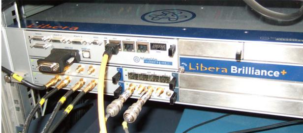
Figure 3: Libera Brilliance+ installation in the TLS with GDX module.
