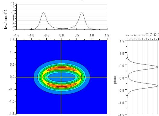
Figure 1: TPS EPU48 synchrotron radiation contour  $K_y = 4$ ,  $K_x = 2.64$  .
