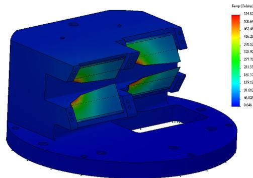
Figure 4: TPS EPU48 XBPM temperature contour when  $K_y = 4$ ,  $K_x = 2.64$ .
