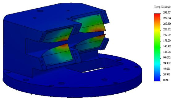
Figure 5: TPS EPU48 XBPM temperature contour when  $K_x = 1.6$ ,  $K_y = 0.8$ .
