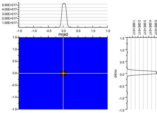
Figure 2: TPS EPU48 first harmonic photon flux contour  $K_y = 4$ ,  $K_x = 2.64$ .
