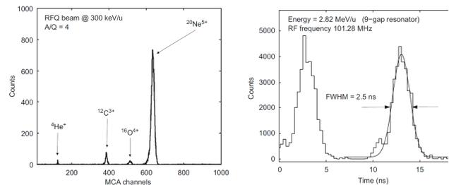
Figure 5: Energy and time spectrum of the Si-det. [4]
