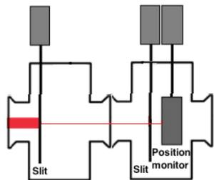
Figure 6: Operating principle of the emittance meter.
