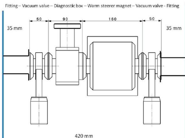
Figure 7: Layout of the inter cryomodule region.
