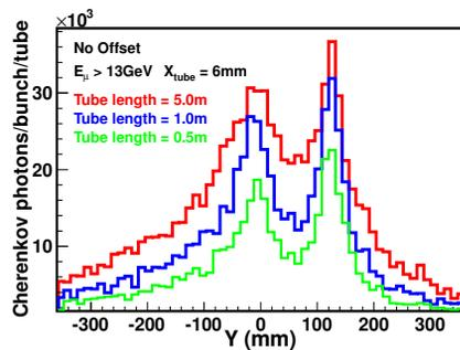
Figure 4: Vertical distribution of Cherenkov photons at the rear window of tubes with  $x = 6$  mm.
