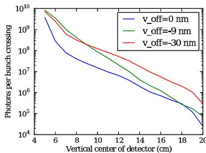
Figure 7: The photon count at a 10 cm photon counter located at 109 m from the IP as a function of the vertical offset of the counter, for three different vertical IP beam-beam offsets.
