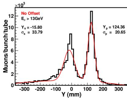
Figure 3: Vertical distribution of the muons entering Cherenkov tubes with  $x = 6$  mm.
