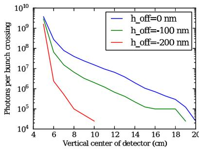
Figure 6: The photon count at a 10 cm photon counter located at 109 m from the IP as a function of the vertical offset of the counter, for three different horizontal IP beam-beam offsets.
