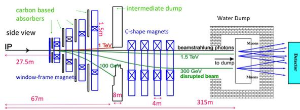
Figure 1: Baseline layout of the post-collision line.
