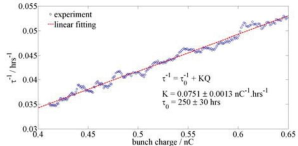
Figure 7: Linear correlation between bunch life and bunch charge.
