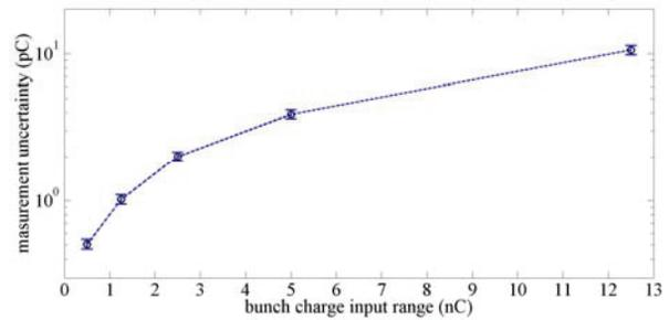
Figure 6: Resolution of bunch charge monitor.
