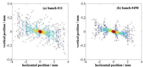
Figure 1: Snapshot of 1650 turns of transverse bunch position after injection.
