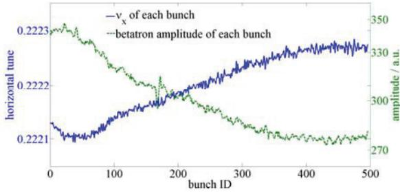
Figure 3: Horizontal betatron tune and amplitude distribution.
