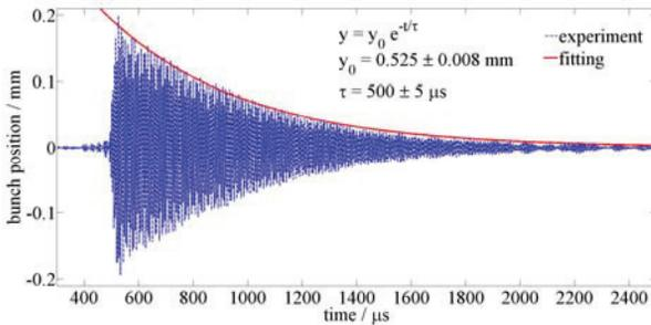
Figure 4: Damping time retrieved from betatron oscillation and fitted envelope.
