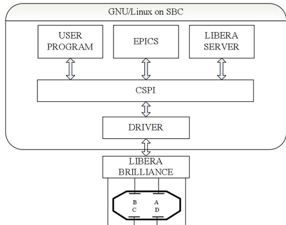
Figure 1: Libera software block diagram.
