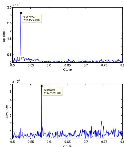
Figure 5: Fractional tune measurement of injection.
