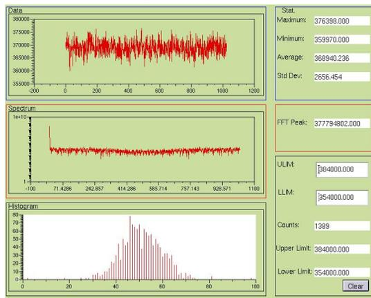
Figure 4: Waveform, spectrum and statistics results.
