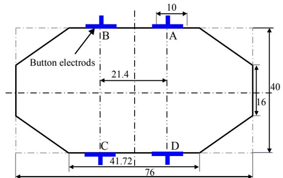
Figure 2: Layout of BPM buttons.
