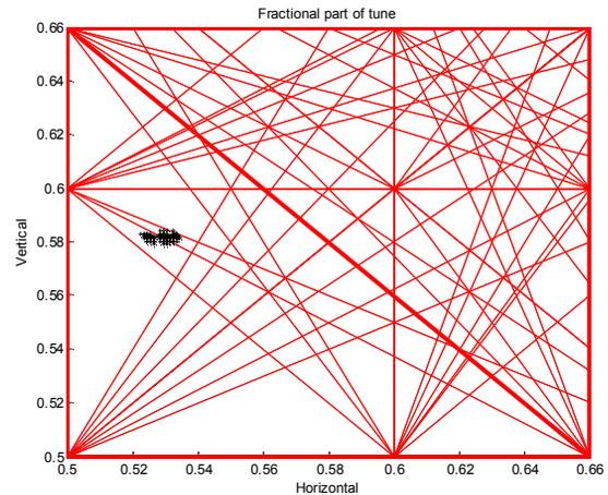
Figure 6: Change of tune during injection.
