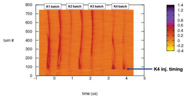
Figure 5: The two dimensional intra-bunch beam loss distribution. A batch is injected from K1 to K4 at intervals of 40ms.
