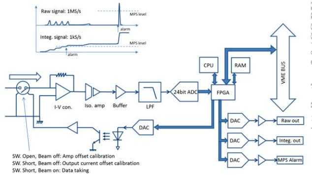
Figure 7: Block diagram of the new data taking system for P-BLM and short-AIC.
