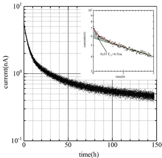
Figure 6: The residual dose measurement using P-BLM after beam stop. The vertical axis shows output current. The enlarged figure is also shown. 1nA output corresponds to 160μSv/h.
