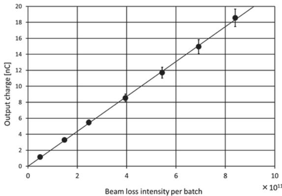
Figure 2: Calibration result of 350BT long-AIC for beam halo/tail monitoring by using intentional beam loss.
