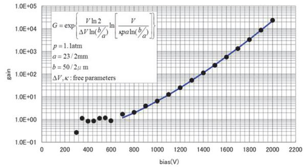
Figure 1: The gain curve of the P-BLM mounted at QM#199. The solid blue line is the fitting result.
