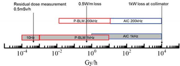
Figure 4: The dynamic range using the both P-BLM and short-AIC. Gas gain of P-BLM is set as  $1E3$ . Open boxes show the dynamic range of the raw signal and the gray boxes show that of integrated signal. The frequency bands of the data are also shown.
