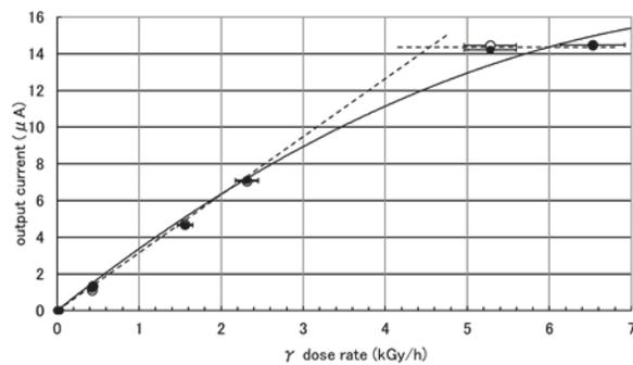
Figure 3: The calibration results of the short-AIC using Co60  $\gamma$  source. The solid circles shows the data of negative biasing to collect negative charged ions and the open circles shows that of positive. The dashed lines are to guide the eyes and the solid line is a fitting result.
